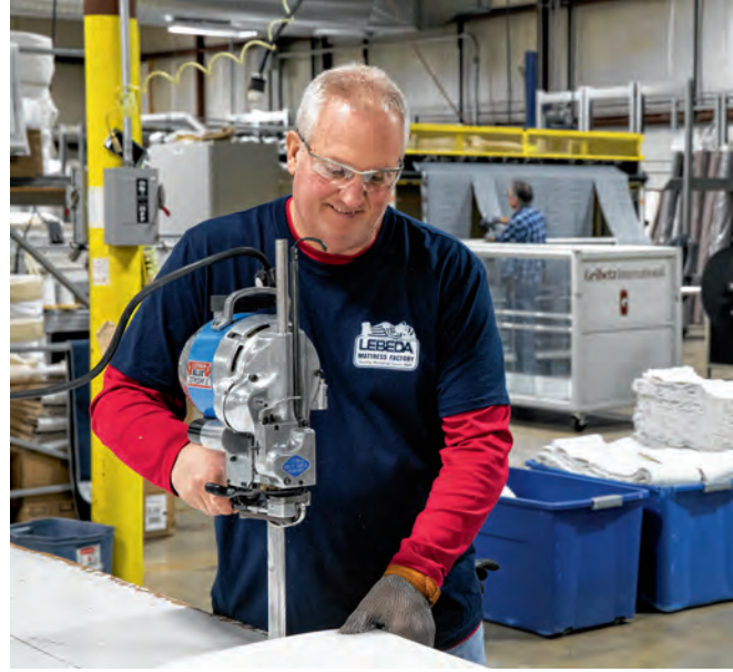
Ron Boots works with an industrial foam cutter to custom cut a piece of mattress foam.
